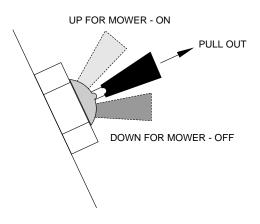
Figure 4-6 Cutter Engage Switch
